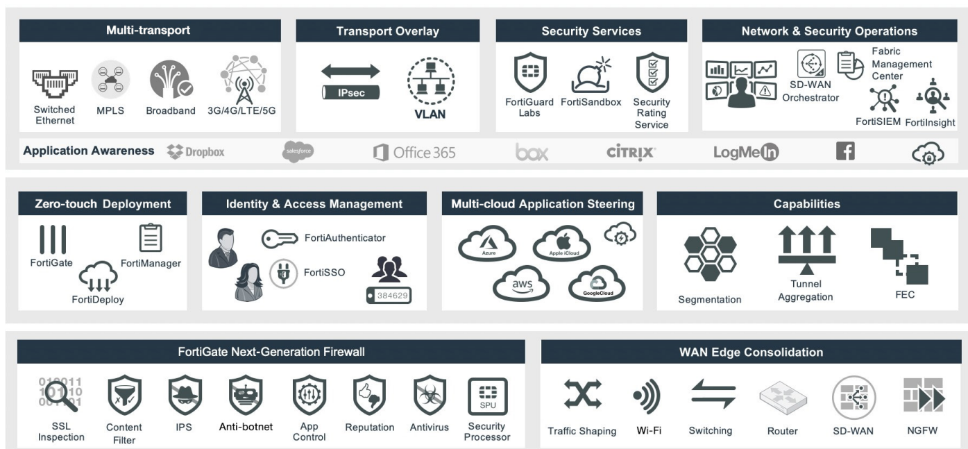
Figure 6. Fortinet Secure SD-WAN architecture components.
