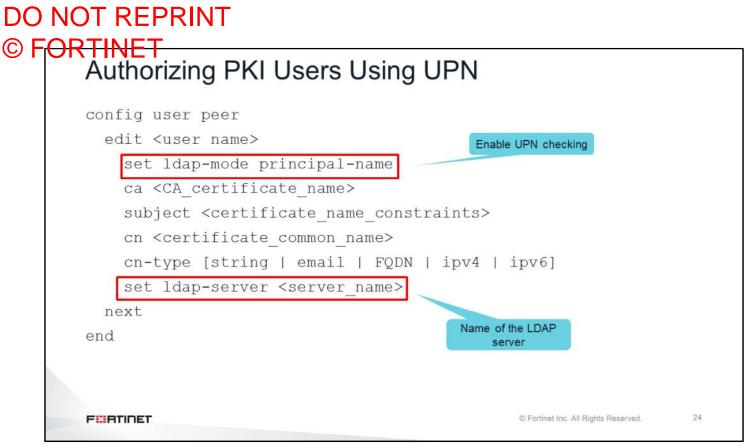
To configure FortiGate to check the UPN in a user certificate, you must change the ldap-mode setting to principal-name. Additionally, you must enter the name of the LDAP server previously configured on FortiGate, that will be used to validate the UPN.
