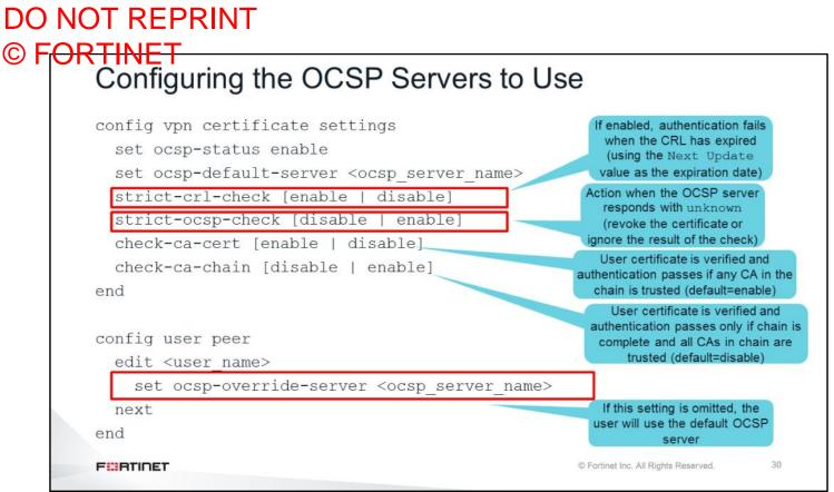
Under config vpn certificate settings, you select which OCSP server (from the previous list) will be the default server used for checking revocation status. You can override that setting per user using the ocsp-override-server setting under config user peer.
