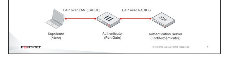
802.1X is a standard that is designed to provide authentication services to network devices that want to join a local wired or wireless network. The 802.1X standard defines an authentication protocol called EAP. It also defines how EAP is encapsulated over the LAN (the EAPOL protocol) and over RADIUS.
