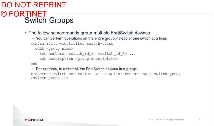
Switch groups, on the other hand, allow you to execute actions over multiple managed FortiSwitch devices. For example, the command execute switch-controller switch-action restart swtp switchgroup restarts all the FortiSwitch devices that belong to the same switch group.
