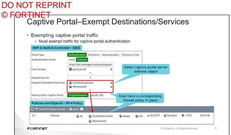
By default, FortiGate blocks all user traffic behind an interface that has the security mode set to captive portal. All HTTP traffic is redirected to the captive portal page and all other traffic is blocked. However, there is an option to exempt certain traffic, allowing it to flow through FortiGate without fulfilling captive portal condition(s) (disclaimer and/or authentication).
