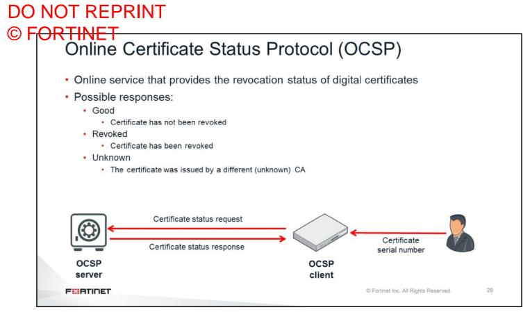
The OCSP offers an online service that provides the revocation status of a digital certificate. Using this protocol, administrators do not need to manually import the CRL into FortiGate. Each time a user presents a certificate, FortiGate uses OCSP to send the certificate's serial number to an OCSP server. The OCSP server replies with one of three possible answers:
