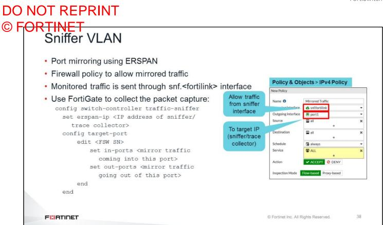
The network traffic sniffer can easily provide monitoring on data traffic passing through FortiSwitch. You can use the predefined sniffer VLAN to use the Encapsulated Remote Switched Port Analyzer (ERSPAN) to monitor traffic sent through the FortiLink sniffer interface.
