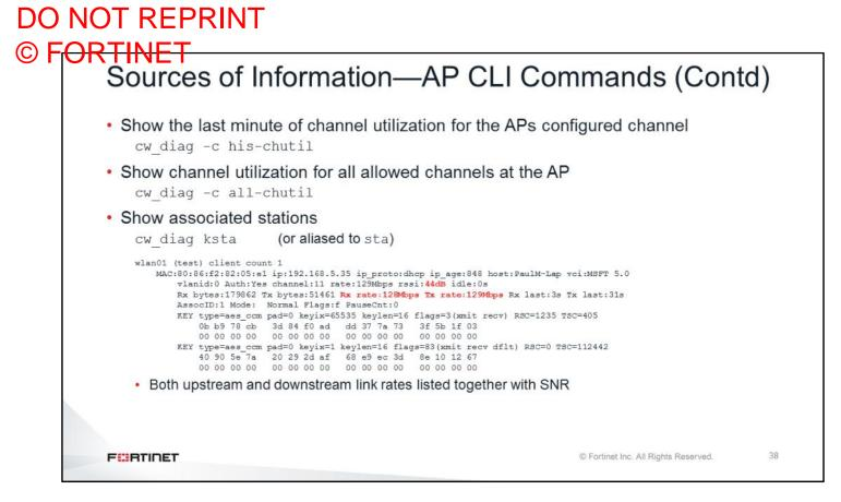
The  $cw_diag -c$  his-chutel command provide a short history of an AP's channel utilization for the AP's radios. So, rather than taking a one-time measure, which could be a peak, you can see over the span of one minute, a plot of the channel utilization.
