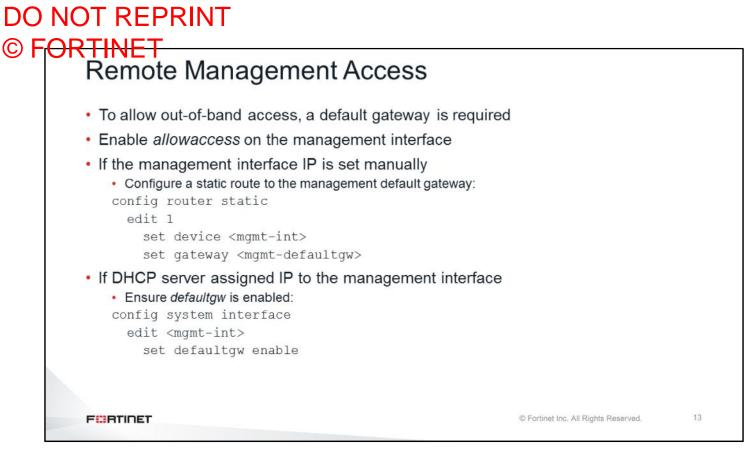
Out-of-band management allows remote access to FortiSwitch. The management interface must enable access using the available management protocol, such as HTTPS and SSH.
