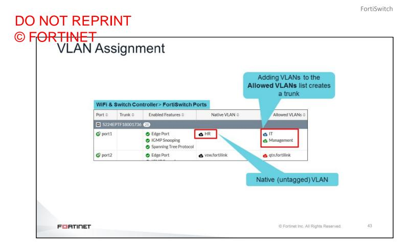
Once you create the VLANs, you define which FortiSwitch ports are assigned to each VLAN by selecting the respective VLAN as the **Native VLAN** for the port. In the same GUI section, you can convert one FortiSwitch port to a trunk by selecting one or more additional VLANs under **Allowed VLANs**.
