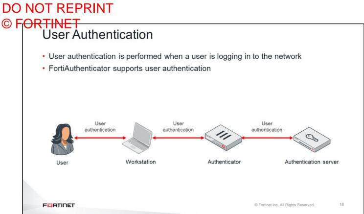
User authentication is performed by a user when that user is logging in to the network.
