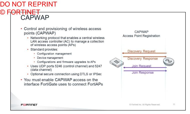
CAPWAP is the network protocol that is used to provision and manage FortiAPs using FortiGate. CAPWAP allows an AC to manage a collection of wireless APs. In the Fortinet Integrated Wireless Solution, CAPWAP enables you to manage configuration, and manage the device, and push firmware upgrades to FortiAPs.
