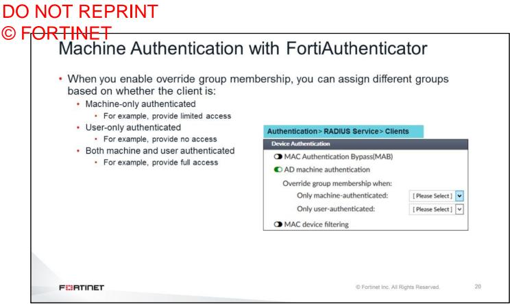
On FortiAuthenticator, you enable AD machine authentication by clicking **Authentication** > **RADIUS Service** > **Clients**. Once you enable AD machine authentication, you can override the user group for clients that have done either machine-only or user-only authentication.
