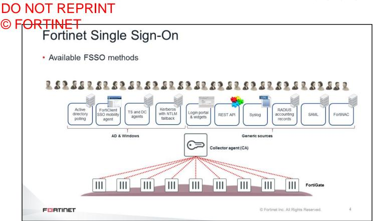
This slide shows the methods you can use to collect sign-on information from, and convert it to, FSSO. You can divide sign-on methods into two groups: Active Directory (AD) and Windows, and generic sources. Sign-on information is sent to FortiAuthenticator, which maintains a record of all the sign-ons learned from different methods and forwards them to FortiGate as FSSO. FortiGate can then use this information to provide accessibility to resources based on FSSO information.
