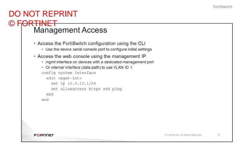
A FortiSwitch device has a serial console port to initially configure the device to allow access through the web console and CLI using an IP address.
