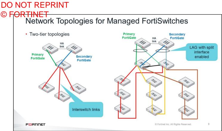
FortiLink supports multi-tier topologies. The example on the left side of this slide shows three FortiSwitch devices connected to one central FortiSwitch. The central FortiSwitch is connected to FortiGate devices in HA mode.
