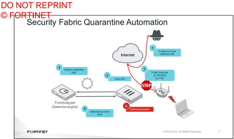
Just like it is with wired clients, known and unknown threat information is easily and efficiently shared among all elements and locations within the Security Fabric. User-defined automation on FortiGate can be used to quarantine compromised hosts; a process that can be strengthened by adding IOC services from FortiAnalyzer.
