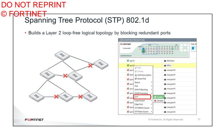
The spanning tree protocol (STP) detects and disables switch ports that create network loops. It automatically builds a network topology free of loops by blocking redundant ports. Switches running STP build this loop-free topology by interchanging bridge protocol data unit (BPDU) frames.
