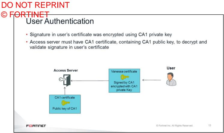
In a similar way, digital certificates can be used to authenticate users. It can be combined with user credentials for two-factor authentication. In this case, when the user is authenticating against an access server, the user sends the digital certificate, which is signed by a CA. The CA signature is encrypted with the CA private key. The access server must have the CA certificate installed (which contains the CA public key) for decrypting and validating the user's certificate.
