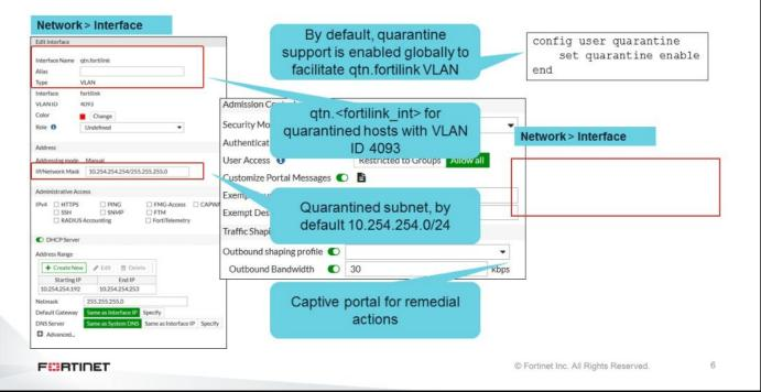
By default, the quarantine VLAN gets created during the FortiLink interface creation process as long as the global setting under the command config user quarantine is enabled on the CLI.
