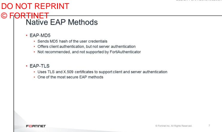
EAP supports multiple methods. There are two types of EAP methods: native and encapsulated.
