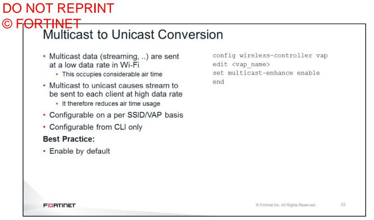
By default, multicast traffic is sent at a lower wireless transmission rate. If a lot of multicast traffic is being passed by the network, then this can needlessly consume airtime.
