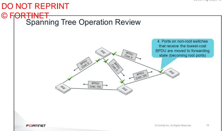
4. Ports in non-root switches that receive the BPDUs with the lowest total-cost-to-the-root value are moved to forwarding state. They become root ports.
