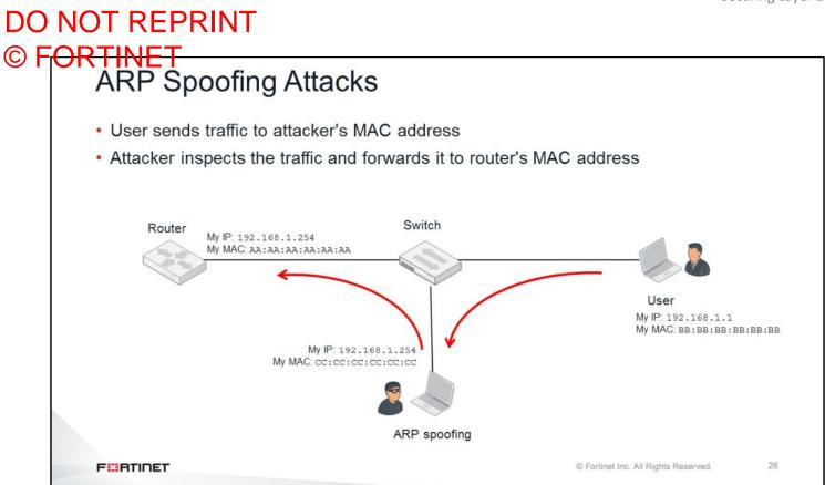
As a consequence of an ARP spoofing attack, all devices start sending traffic destined to the spoofed IP address to the attacker's machine. The attacker can then inspect and potentially modify the traffic before forwarding it to the device that legitimately owns the spoofed IP address.
