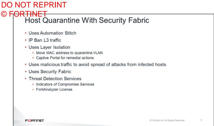
When a FortiGate is a member of a Security Fabric group, the Security Fabric an quarantine hosts automatically using Security Fabric automation stitches. If you are using IP ban and access layer isolation, then place the host into a quarantine subnet, which is created by default when you create a FortiLink interface.
