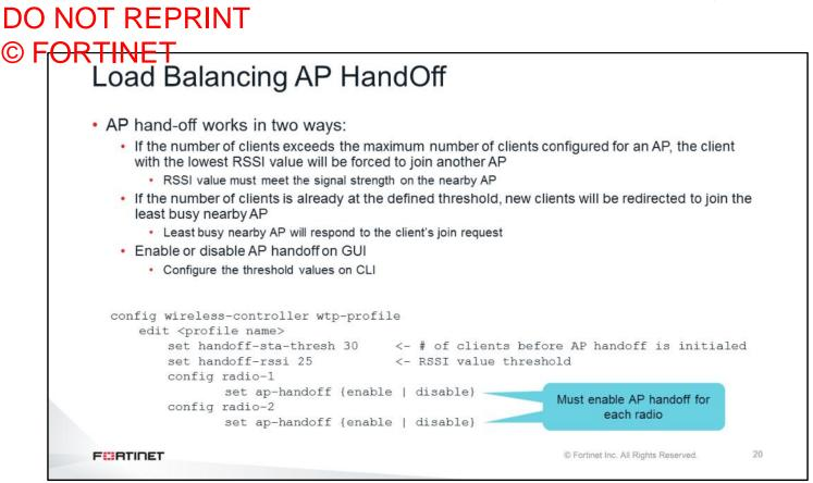
AP handoff is a load balancing method that is used by FortiGate to increase wireless performance and use the resources on APs more efficiently. AP hand off is a way of load balancing wireless clients among managed APs on FortiGate. If an AP is overloaded and the maximum number of clients is configured for an AP or radio, FortiGate will drop the client that has weakest signals and connect the client to a nearby AP.
