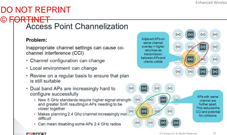
A big source of issues with a wireless network can be incorrect channel setting.
