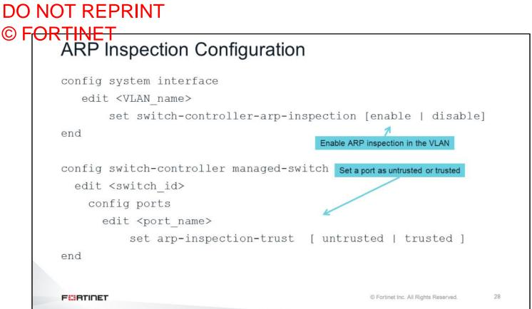
ARP inspection is enabled at the VLAN level. Each port is then configured as trusted or untrusted.
