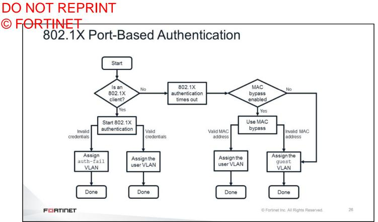
This slide shows the authentication process when 802.1X is combined with MAC address bypass. When a physical device is connected to an 802.1X port, FortiSwitch waits for the EAPOL-Start packet.
