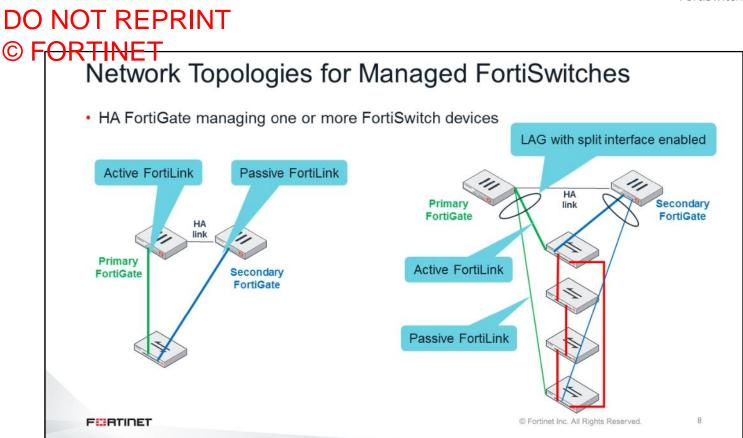
The example on the left side of this slide shows a deployment with two FortiGate devices in HA mode, and one FortiSwitch. The primary FortiGate has the active FortiLink. The secondary FortiGate has the passive FortiLink.
