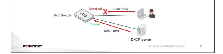
DHCP snooping inspects DHCP traffic in order to build a table that contains the MAC address, assigned IP address, and port number for each DHCP client.
