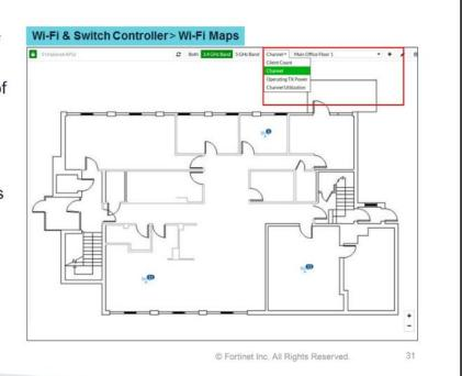
It is often difficult to work out from a static table how an AP location will relate to another. The location of an AP is particularly important when assessing the channel setting, and using the Wi-Fi map will allow you to identify adjacent APs that might, for instance, have the same channel number, potentially causing an issue.
