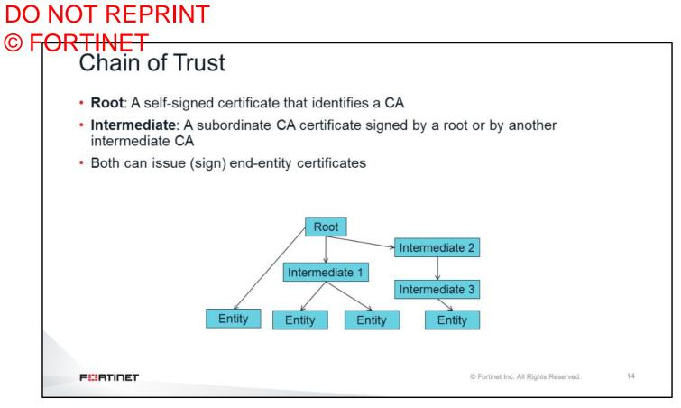
Digital certificates are validated through a chain of trust. The simplest chain of trust occurs when the root CA is directly signing the end-entity certificates. However, a chain of trust can include one or more intermediate CAs. Both root and intermediate CAs can sign end-entity certificates.
