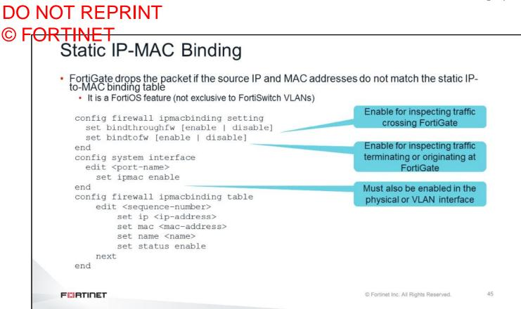
DHCP snooping dynamically creates an IP-to-MAC binding table. You can also create a static IP-to-MAC binding table with these commands. This is a FortiOS feature that you can use with or without FortiSwitch. FortiGate drops the packet if the source IP and MAC addresses do not match the information in the static IP-to-MAC binding table.
