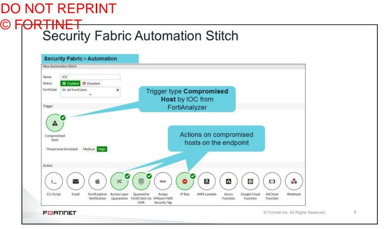
Compromised wireless hosts are treated in the same way as compromised wired hosts; FortiAnalyzer identifies them using threat detection services, and then sends the IOC verdict to the root FortiGate of the Security Fabric group.
