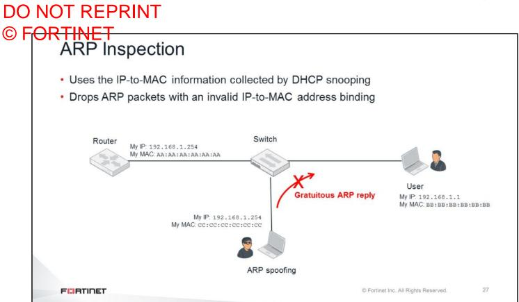
ARP inspection can prevent ARP spoofing attacks. ARP inspection uses the IP-to-MAC binding table populated by the DHCP snooping feature, to drop invalid ARP packets. An ARP packet is categorized as invalid when the IP and MAC address pair does not match the information in the IP-to-MAC binding table.
