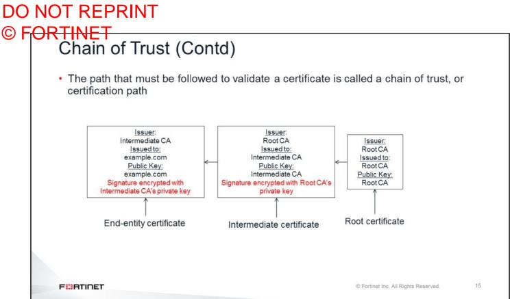
In the example shown on this slide, the end-entity certificate was signed by an intermediate CA. The intermediate CA certificate was signed by the root CA.
