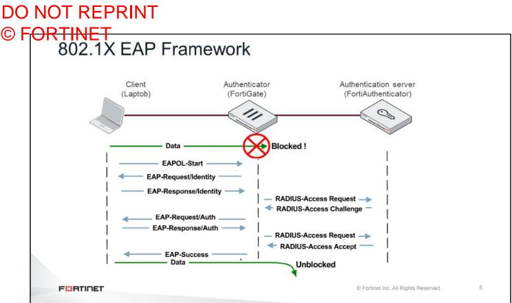
When a supplicant client (laptop) connects to a LAN switch that requires 802.1X authentication, the client credentials are sent to the authenticator (FortiGate), using EAP over LAN (or EAPOL). The authenticator (FortiGate) then forwards the EAP traffic to the authentication server (FortiAuthenticator), which is an EAP over RADIUS server.
