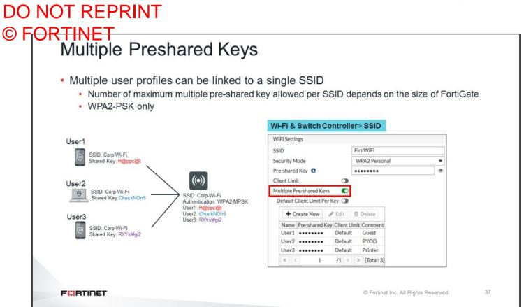
As an extension to the original PSK standard, it is possible to enable multiple PSKs for a wireless network. This allows multiple keys to be used to allow access to the network, making key management easier, because all users and devices have unique credentials. If a user leaves or a device is lost, the multiple preshared keys credential is simply changed for that one user or device.
