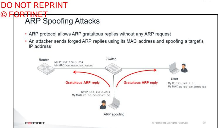
A security weakness in the ARP protocol is that it allows devices to send ARP replies without any ARP request. These packets are called gratuitous ARPs. This weakness can be exploited to execute an ARP spoofing attack (also called an ARP poison attack).
