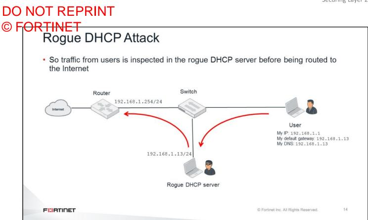
After the rogue DHCP server assigns the malicious default gateway and DNS, attackers start receiving clients' traffic. Attackers can also manipulate the DNS replies to redirect client traffic to malicious external destinations.
