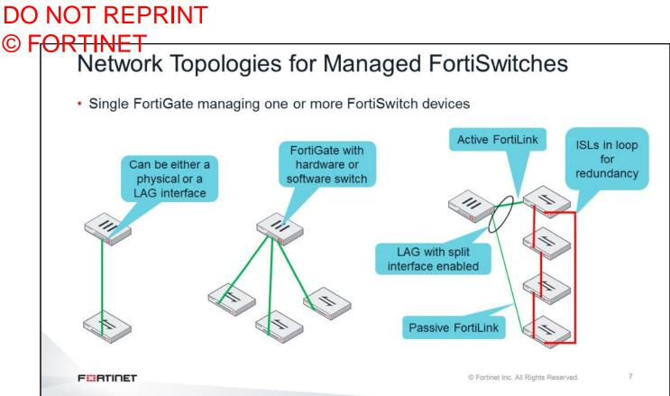
Now, you will learn about the different ways you can deploy FortiSwitch using FortiGate. The simplest deployment is one FortiGate managing one FortiSwitch. The interface FortiGate uses to manage FortiSwitch could be either one single physical interface, or an aggregated interface with multiple physical interfaces.
