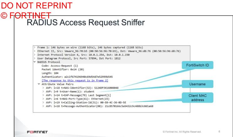
This packet capture shows the RADIUS Access-Request that is sent from a Layer 2 switch (acting as an authenticator) to the authentication server. It contains the switch ID, username, and switch MAC address.
