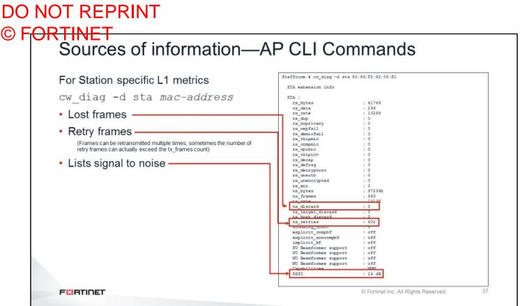
For stations, you can list more detailed RF information by using the  $cw_diag -d sta$  command for a specific station MAC address.
