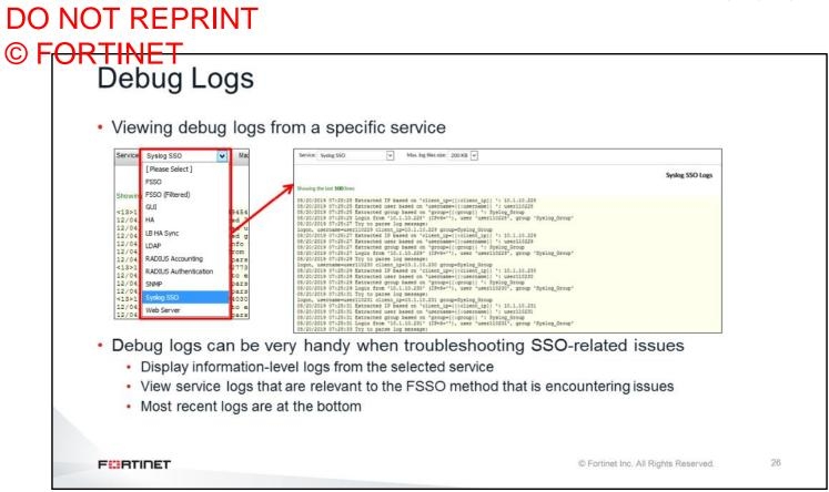
You can also view SSO-related logs that are specific to a single SSO source, such as RADIUS accounting or the Syslog feed. For example, you can view the RADIUS attributes that are sent in the accounting message, or view the raw Syslog feed that FortiAuthenticator is receiving.
