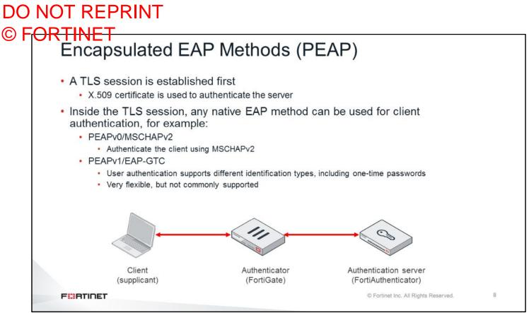
With encapsulated EAP methods, a TLS session is established first. At this point, a digital certificate is used to authenticate the server. Encapsulated inside the TLS session, any native EAP method is used for client authentication. Two examples of encapsulated EAP methods are:
