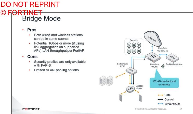
In local bridge mode SSID, wireless traffic is bridged directly to the local LAN that the AP is connected to. This mode is useful when deploying APs, at remote locations, that connect to a wireless controller over a WAN link. To ensure all traffic is scanned for security threats, consider deploying smart-series APs in this type of deployment.
