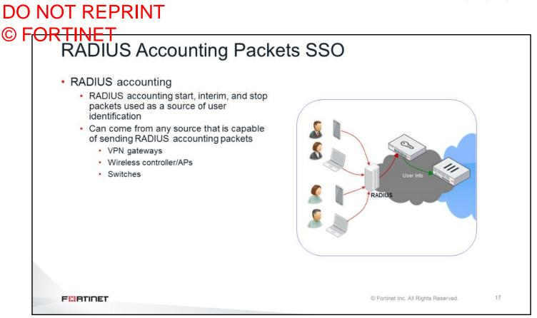
The RADIUS accounting method uses RADIUS start, interim, and stop accounting packets to trigger logon and logoff events to FSSO. Such RADIUS packets are commonly sent by networking devices such as SSL-VPN devices, wireless controllers, switches, and so on.
