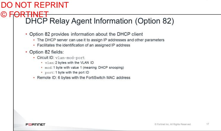
DHCP snooping can optionally insert the DHCP option 82 field into the DHCP packets coming from the clients. The option 82 field contains the VLAN ID, port ID, and FortiSwitch MAC address. This information can help administrators to locate the devices in the network. Additionally, the DHCP server can use this information to make assignment decisions based on the location of the device.
