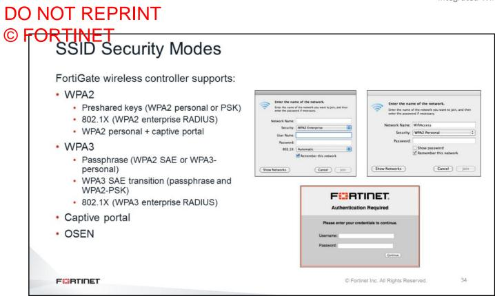
Configuring the profile requires the setup of the security mode. Security modes are settings for client authentication and traffic encryption between the wireless client and the AP. Remember, wireless is a shared medium, so there are even more vectors of attack than for wired connections. The FortiGate wireless controller supports multiple authentication methods:
