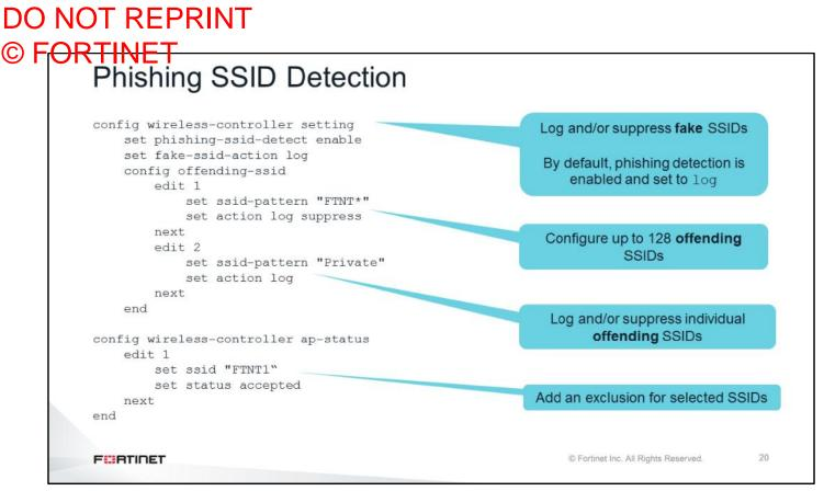
Currently, you can configure phishing SSID detection only using the CLI. By default, fake SSIDs are only detected and logged.
