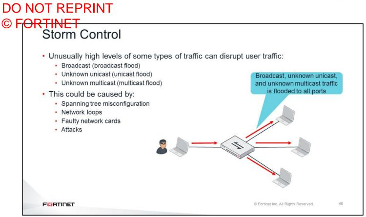
A Layer 2 storm is an usually high level of some type of traffic that can disrupt user traffic. The types of traffic that could potentially create storms are broadcast, unicast to invalid destinations (unknown unicast), and multicast to invalid destinations (unknown multicast).
