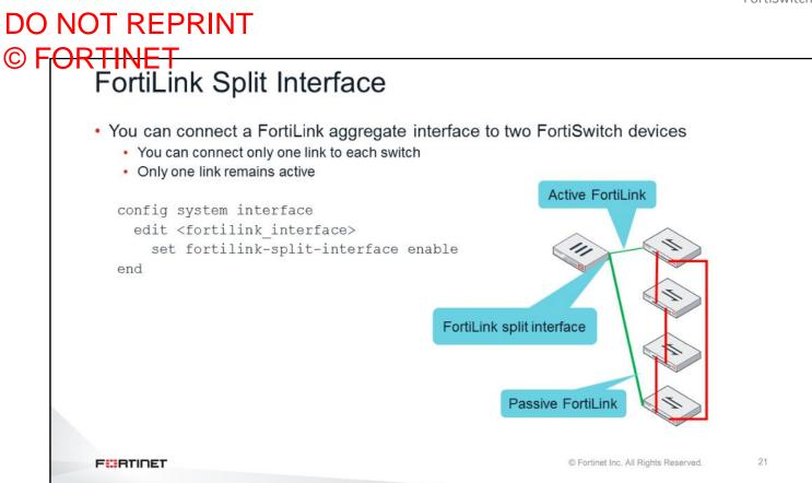
As you learned earlier, you must enable a split interface on a FortiGate aggregated interface to allow two links to be connected to different FortiSwitch devices. One link will be active, the other one will be inactive. This is required in some deployment modes, like the example shown on this slide, which shows multiple FortiSwitch devices connected in a ring topology.
