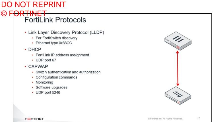
FortiGate uses multiple protocols for discovering, provisioning, and administrating FortiSwitches. First, FortiGate uses the Link Layer Discovery Protocol (LLDP) to discover FortiSwitch. After that, and after FortiSwitch is authorized, DHCP assigns the FortiSwitch IP address. After IP connectivity is up, CAPWAP authenticates and authorizes the switch. FortiGate also uses CAPWAP to carry configuration commands, monitoring, and software updates.
