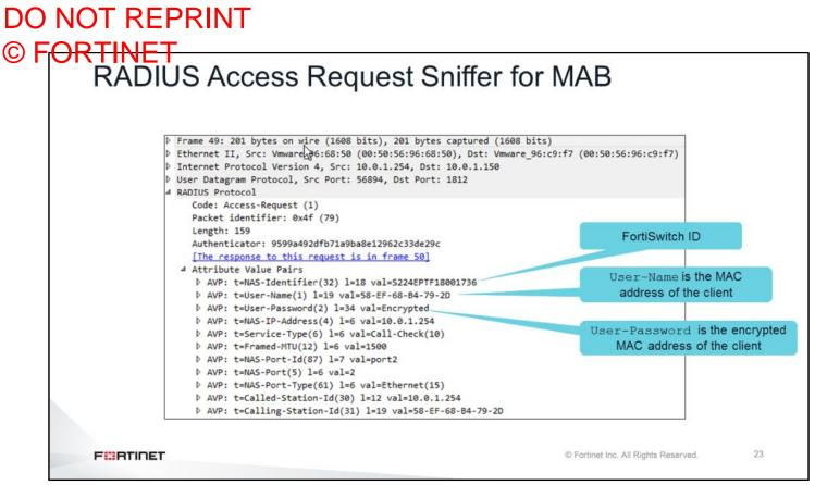
This packet capture shows the RADIUS access request when MAB is used. It includes the FortiSwitch ID, client MAC address (as the username), encrypted client MAC address (as the password), and the client MAC address (as the Calling-Station-ID).
