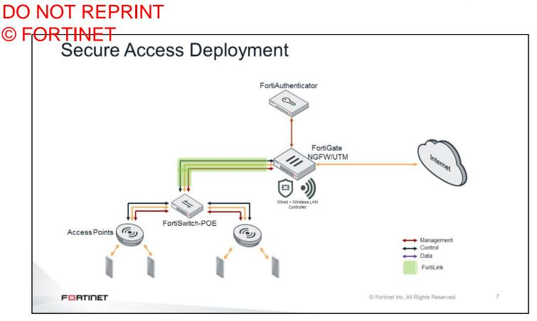
Fortinet's Secure Access solution includes APs, switches, and a firewall. This slide shows a high-level deployment diagram.
