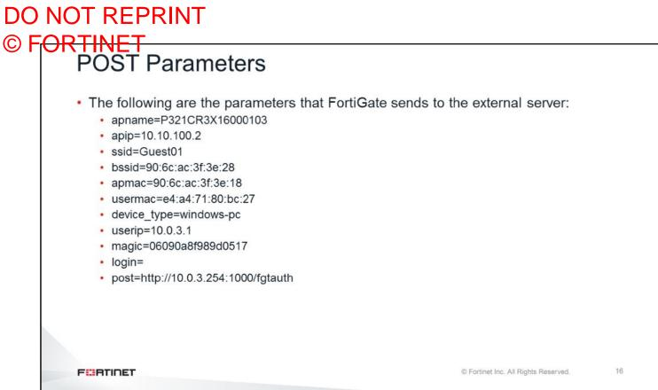
This slide contains a list of all the parameters that are sent to the external captive portal from a wireless network on FortiGate.
