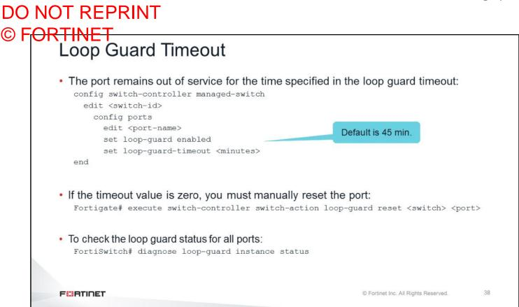
When loop guard detects a loop, the loop guard timeout defines the time the port will remain shut down.
