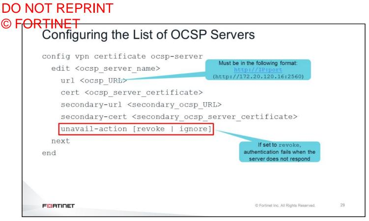
You can configure FortiGate with a list of OCSP servers that can be used to validate the revocation status of user certificates. For each OCSP server, you configure its URL and the CA certificate (cert) of the CA that signed the OCSP certificate (this is used for authenticating the OCSP server). Optionally, you can configure a secondary (backup) OCSP server, for cases where there is no reply from the primary server.
