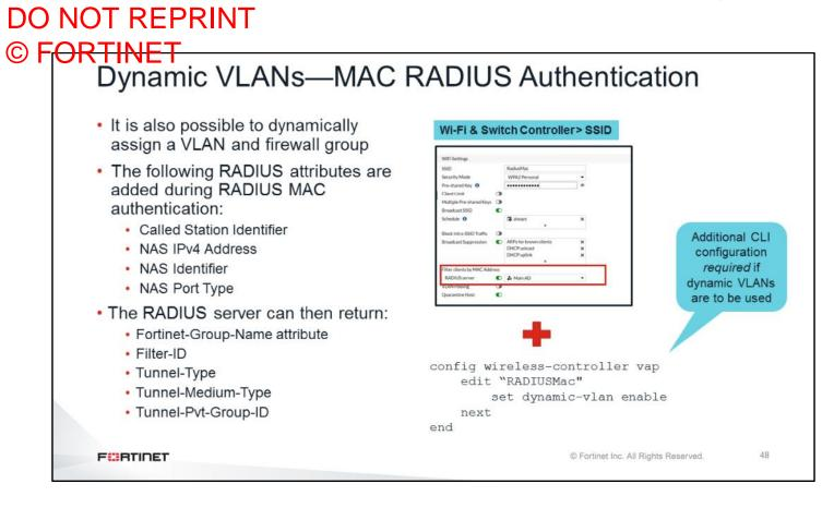
It is also possible to add dynamic VLANs to a non-enterprise network. Traditionally, open or preshared key networks did not allow for the dynamic allocation of VLANs. But, MAC filtering using RADIUS, it is now makes it possible to pass back the following attributes to the RADIUS server when authenticating clients using their MAC addresses:
