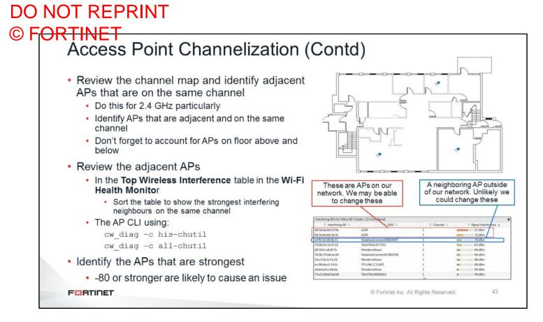
When reviewing the AP channels, the Wi-Fi map is very useful. It allows you to view the channel settings for each AP, instantly seeing which AP interfaces could be interfering with each other. It is possible to view each frequency individually. You should pay particular attention to the 2.4 GHz interfaces, because these are the ones that usually experience issues.
