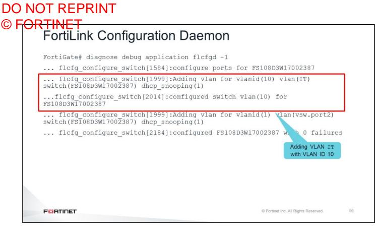
The output of the real-time debug for the flcfgf process provides information about configuration changes pushed from FortiGate to FortiSwitch. In the example output shown on this slide, an administrator has created a new VLAN named IT, with tag ID 10. The output shows the moment when FortiGate pushed this new VLAN configuration to FortiSwitch.
