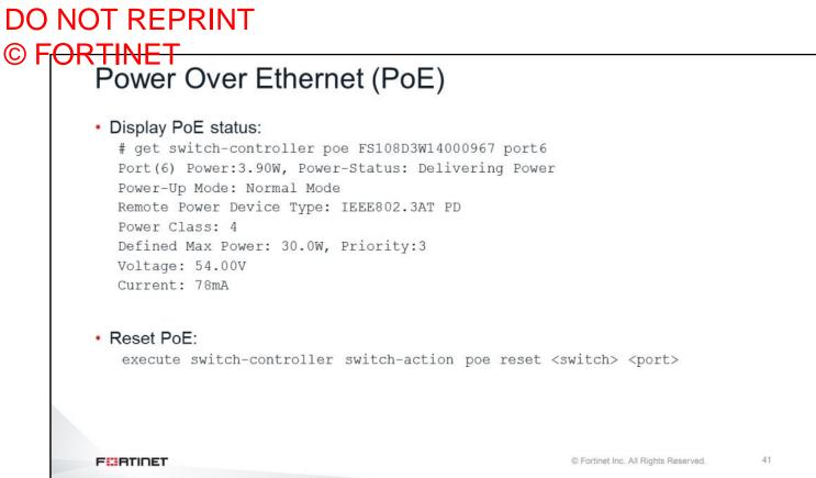
You can also restart the port PoE on the CLI, using the command execute switch-controller poereset.
