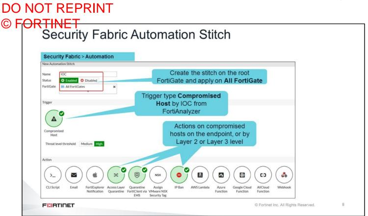
Compromised hosts are identified by FortiAnalyzer using Threat Detection Services. IoC verdicts get sent to the root FortiGate of the Security Fabric group in order provide the required information in case there is an Automation Stitch configured for compromised hosts.
