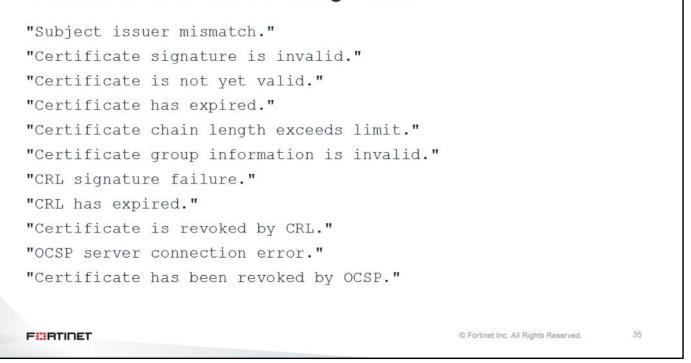
If there is any problem during the validation of a user's certificate, the output of the non-blocking authentication real-time debug will display an error explaining why the certificate validation failed. The possible reasons are listed on this slide. Some of them include:
