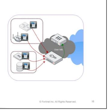
FortiAuthenticator can also parse username and IP address information from a Syslog feed from a third-party device, and inject this information into FSSO so it can be used in FortiGate firewall policies. You can use the Syslog feed to trigger logon, update, or logout rules on FortiAuthenticator. You can use any Syslog server to send the username and IP address information to FortiAuthenticator, as long as you have configured a corresponding matching rule.
