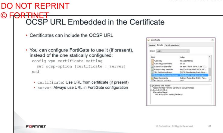
In some cases, the user certificates contain the URL of an OCSP server that can be used to check the revocation status. You can configure FortiGate to either use this information (if available in the certificate), or ignore it (and keep using the OCSP server configured in the FortiGate configuration).
