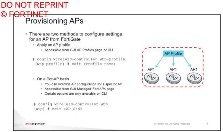
FortiGate automatically assigns a *default* AP profile to an AP when it is discovered and manually authorized. Once a CAPWAP tunnel is established between a FortiGate and an AP, the FortiGate uses the CAPWAP control channel to push all AP profile parameters to the AP.
