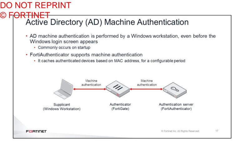
In Windows environments, there are two types of 802.1X authentication: AD machine authentication, and user authentication.
