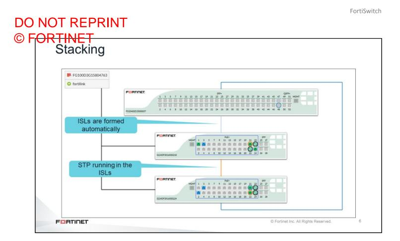
Using FortiLink, FortiGate automatically provisions stacked FortiSwitches, forms inter-switch link (ISL) between FortiSwitch devices, and enables the Spanning Tree Protocol on the ISLs. FortiGate autodiscovers all FortiSwitch devices in the stack, and manages them centrally.
