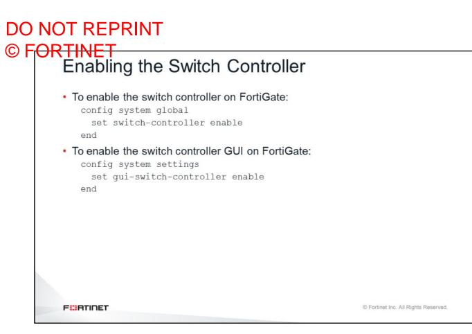
By default, the FortiSwitch controller is disabled. You must enter the config system global command followed by the set switch-controller enable command.
