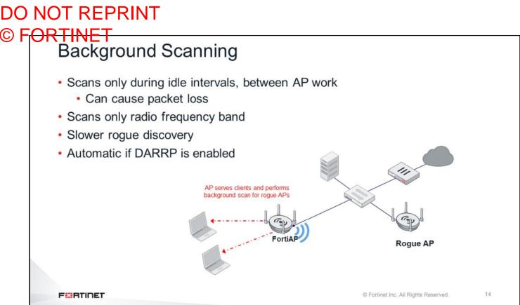
How does rogue AP detection on FortiOS work? It uses a radio to listen for, and detect, other APs. If your FortiAP is not using all of its radios, you can dedicate one of them to monitoring for rogue APs. Otherwise, you can configure the AP to run a background scan when a radio is idle.
