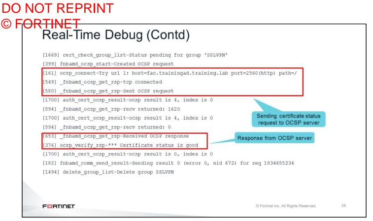
In the example shown on this slide, FortiGate is configured to validate the certificate revocation status using OCSP. The output of the real-time debug shows the OCSP URL and a log entry indicating that the OCSP request has been sent.
