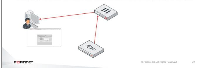
FortiAuthenticator uses the provided POST parameters and RADIUS client configuration to search the mapping rules. If all the conditions defined in a mapping rule are met, FortiAuthenticator uses the mapped guest portal and presents the login page to the user.
