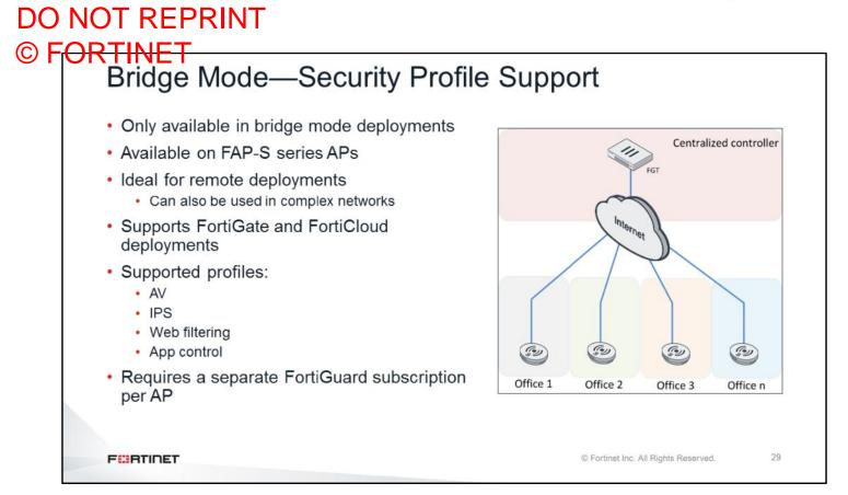
If a bridge mode SSID is configured for a managed FortiAP-S (or smart FortiAP), you can add a security profile group to the wireless controller. This configuration allows you to apply the following security profile features to the traffic over the bridge SSID:
