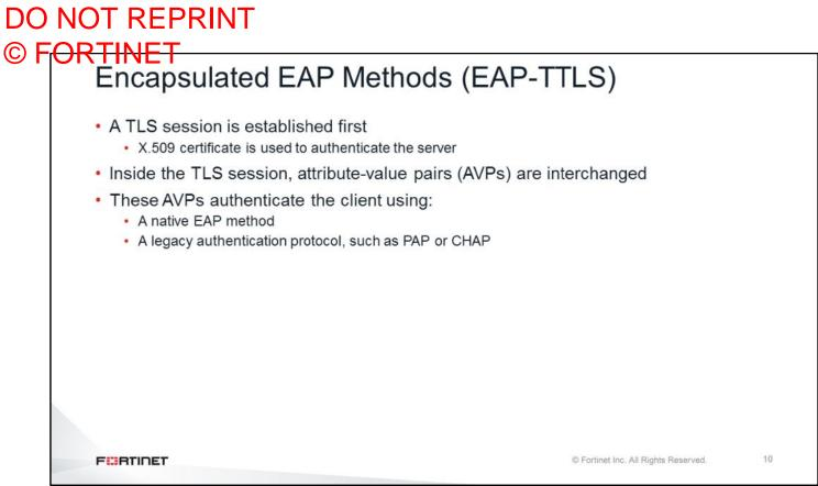
Another encapsulated method is EAP tunneled TLS (EAP-TTLS). With this method, attribute-value pairs (AVPs) authenticate clients using either a native EAP method or a legacy authentication protocol (such as PAP or CHAP).
