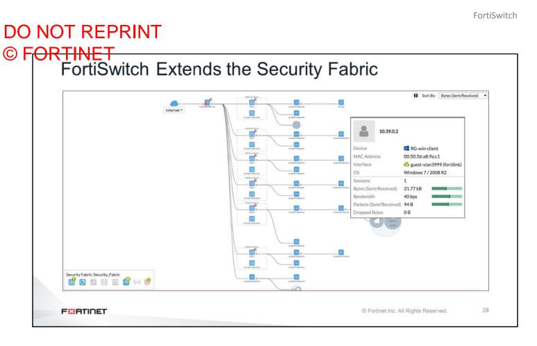
A managed FortiSwitch is an extension of a FortiGate device. In this way, FortiSwitch extends the visibility of the Fortinet Security Fabric up to Layer 2. Using FortiView physical and topology views, you can visualize different security segments, together with all the stacked FortiSwitch and end devices connected.
