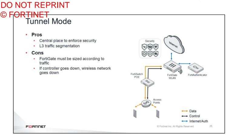
By default, tunnel mode SSID is selected when you define an SSID on FortiGate. In this mode, all traffic within CAPWAP DTLS or non-DTLS tunnels is sent to FortiGate before it is allowed on the LAN or the Internet. There are two main advantages to using this mode:
