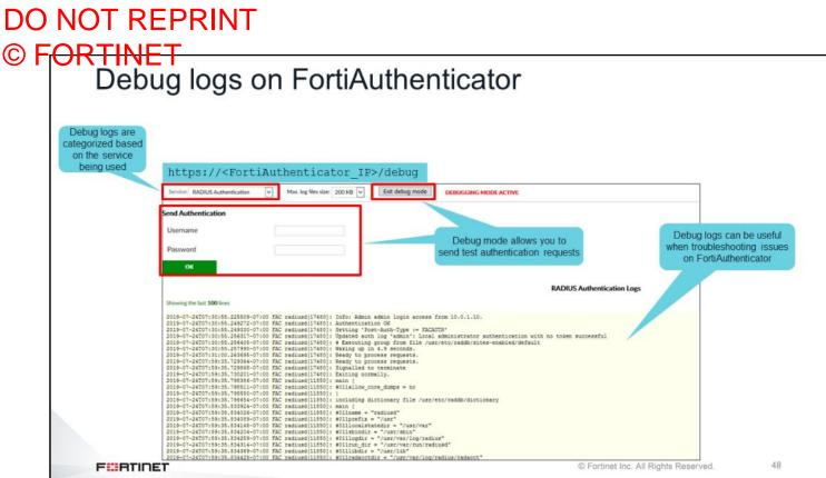
Unlike FortiGate, FortiAuthenticator does not have real-time debug commands. Instead, you can access extended logs for individual services. You can access the debug log page using the URL at <a href="https://<FortiAuthenticator\_IP>/debug">https://<FortiAuthenticator\_IP>/debug</a>. These logs can be used to troubleshoot issues with services running on FortiAuthenticator.
