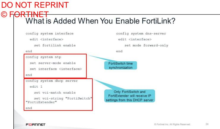
When you dedicate a FortiGate interface to FortiLink, the system automatically applies the following configuration changes to the FortiGate configuration:
